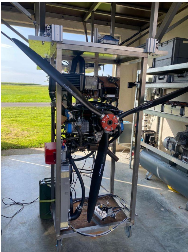
Figure 1: 'Smart propeller' on the drive test bench at Helix Carbon
