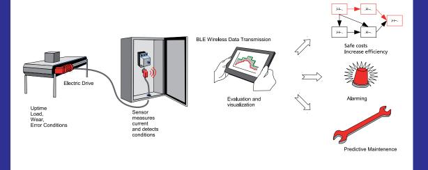
And smart data processing enables deduction of high number of single sensors. The determination of mechanical and electrical conditions can be done by the analysis of the supply current. Switching states of control elements, torque on electric motors leads to characteristic supply currents. By measuring the supply current and doing suitable signal processing the mechanical state can be determined.
