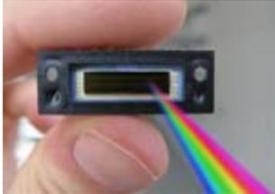
Image sensors as used in cell phones are partially color-blind. This is because of their coating, which prevents UV light from passing through. CMOS chips have as a result not been suitable for spectroscopy up to now. A new production process makes the coating transparent – and the sensors suitable for special applications.
