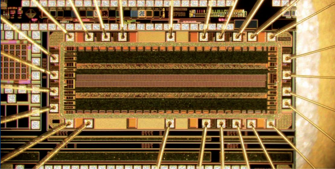
Integration of tailored CMOS readout electronics on the same chip allows adaptation of the sensor performance according to the requirements of the intended applications. The SPADs can be used as 1D or 2D arrays and, by integration of quenching resistors on the pixel level, even as silicon photomultipliers (SiPM).
