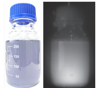
Image of purified (6,4)-SWCNTs (left) and fluorescence image of the SWCNTs in the NIR. © Fraunhofer IMS
