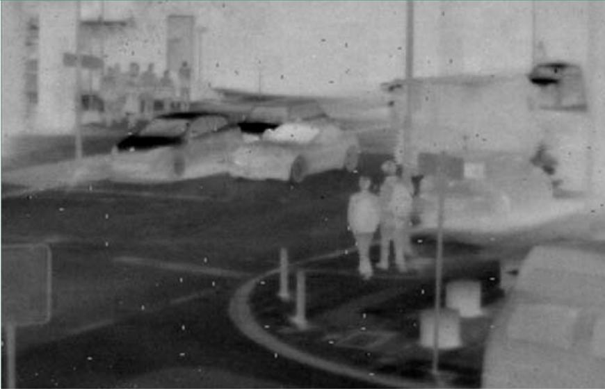
Infrared imagers »see« in a wave length range from the near up to the long-wave infrared. These thermal image sensors are called focal plane arrays and are one- or two-dimensional lines of IR-sensitive pixels. They are based on radiation-sensitive structures on silicon technology, where CMOS read-out circuits are integrated on a chip. That's how complete image sensor chips are developed.
