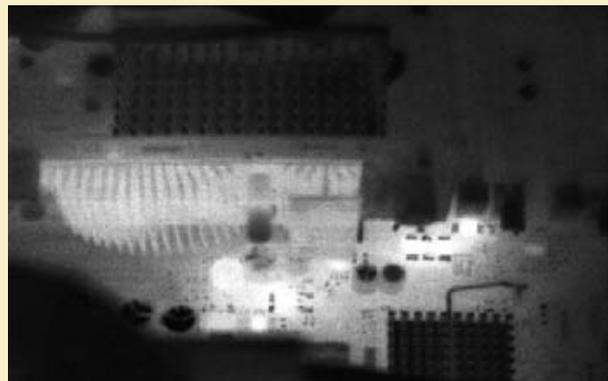
Figure 6: Uncompensated IR image of a PC main board
