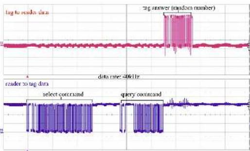
Figure 4: Measured data signals during wireless communication at 40 kHz. (Digital part for ISO/IEC protocol handling implemented on FPGA with separate power source)
