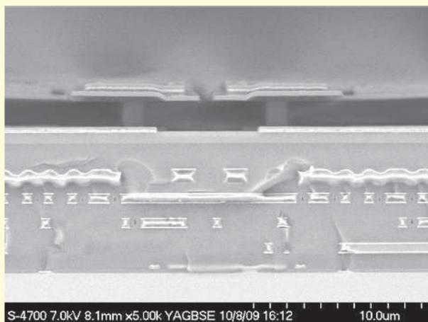
*Figure 2: Microbolometers on top of CMOS readout*
