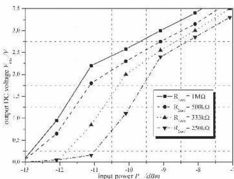
Figure 6: Measured output voltage for different load currents
