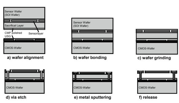
Fig.7: Process flow for the fabrication of a diode bolometer
