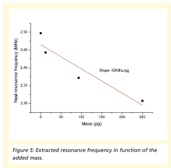
Figure 5: Extracted resonance frequency in function of the added mass.
