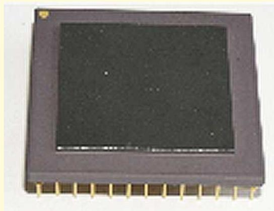
*Fig.12: Ceramic vacuum package after lid soldering*
