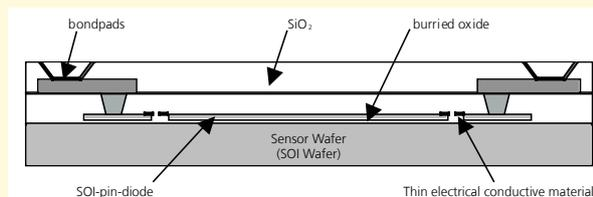
Fig.1: Cross section of a SOI-pin-diode test structure
