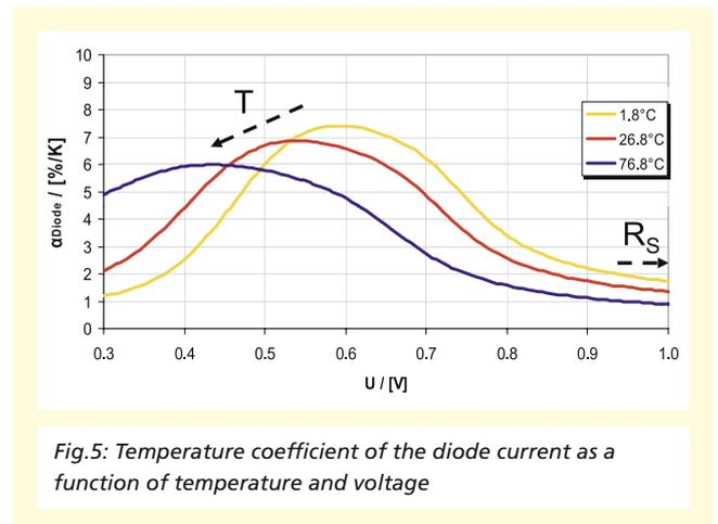
Fig.5: Temperature coefficient of the diode current as a function of temperature and voltage
