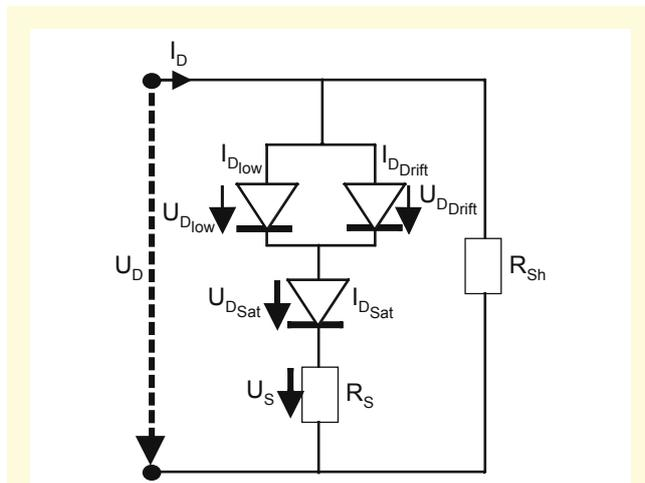
Fig.3: Temperature dependent DC-model for a SOI-pin-diode test structure and diode bolometer
