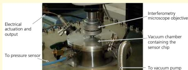
*Figure 3: Measurement set-up for the proof of concept experiment showing the sample chamber with the inlets for electrical actuation and pressure monitoring. The interferometry microscope measures the deflection of the membrane through a glass window.*
