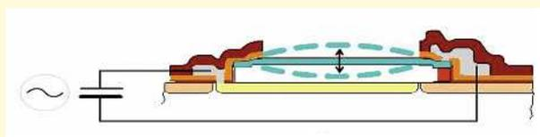
*Figure 1: Schematic cross section of the sensor. The poly-silicon membrane is depicted in blue and the bottom substrate electrode in yellow. The sensor is excited with a sine signal with an offset.*
