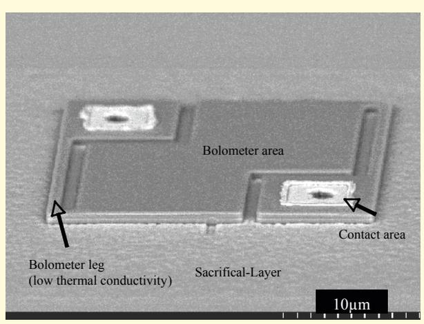
Fig.9: Diode bolometer before release step
