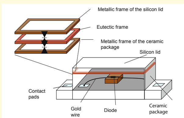
*Fig.11: Schematic illustration of a vacuum package*
