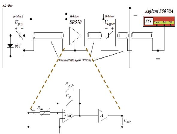
Fig.6: Noise measurement setup for noise determination of diodes
