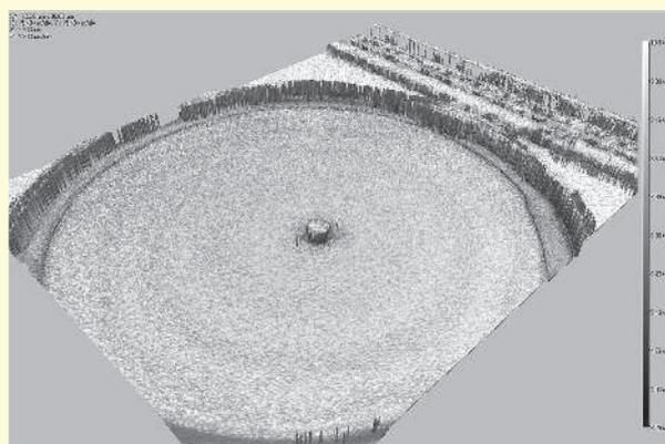
*Figure 2: Optical interferometry image of a  $\text{SiO}_2$  post deposited in the middle of a membrane of about  $96 \mu\text{m}$  in diameter.*
