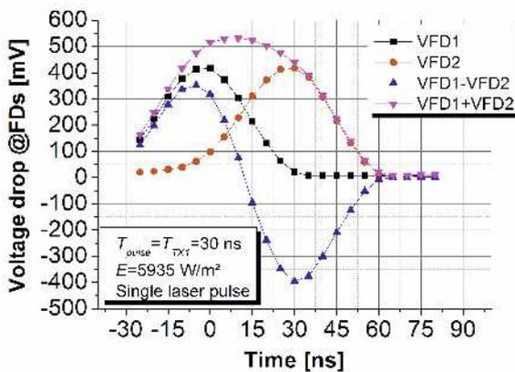
Figure 6 Time-of-Flight operation of a LDPD structure.
