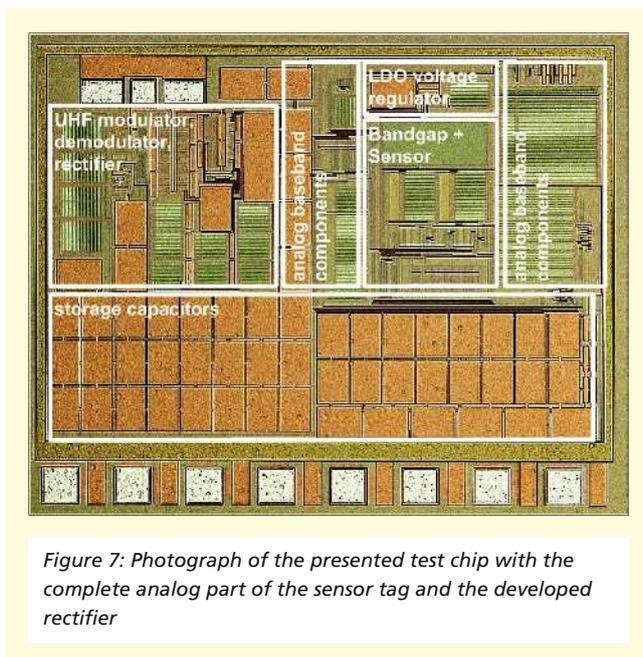
Figure 7: Photograph of the presented test chip with the complete analog part of the sensor tag and the developed rectifier
