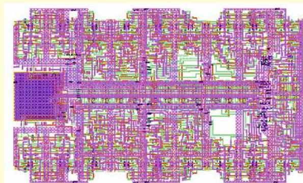
*Fig. 2: Full-Custom Layout of the Sinc Filter Datapath. Vertical control and power tracks in metal 3 and 4 layers are not shown.*
