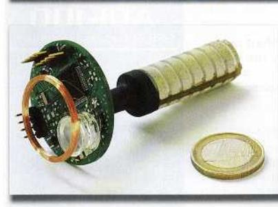
The passive sensor-transponder continuously monitors the protective coating of concrete bridges, allowing corrosion damage to be detected at an early stage. Image courtesy of Fraunhofer IMS.
