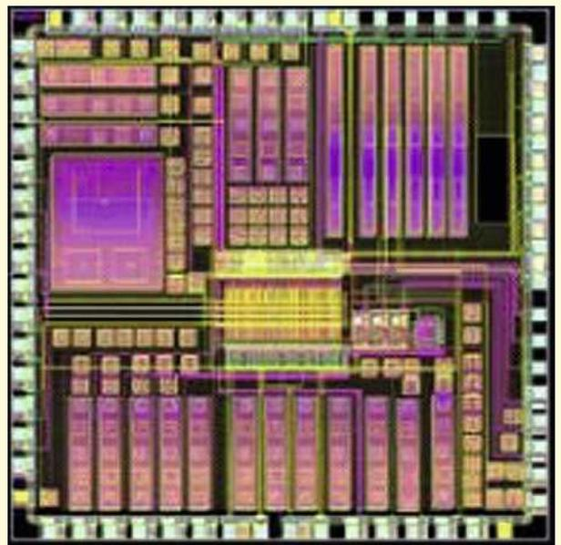
Figure 7 Layout of a 3D ToF test chip with PG, PPD and LDPD pixels.
