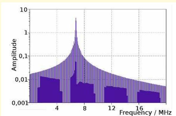
Fig. 6. Spectrum of antenna voltage using load-modulation
