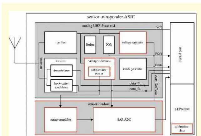
Figure 1: Architecture of a transponder with additional circuitry for temperature measurement.
