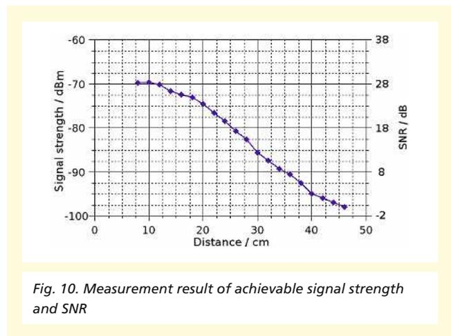
Fig. 10. Measurement result of achievable signal strength and SNR
