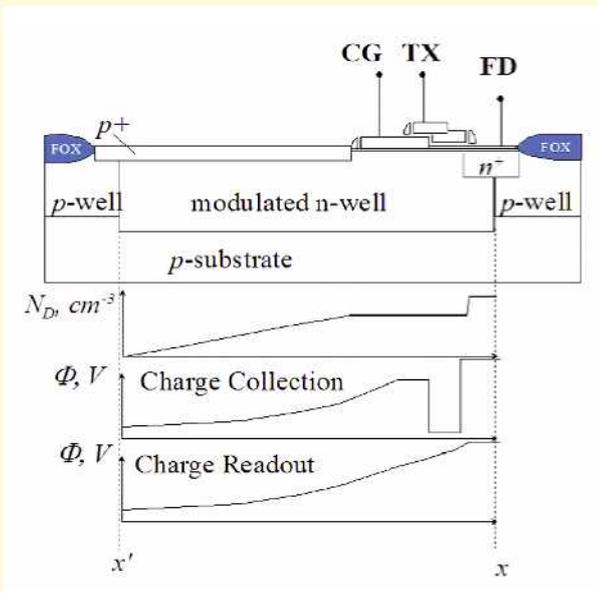
Figure 3 Layout of a lateral drift-field photodiode (LDPD).
