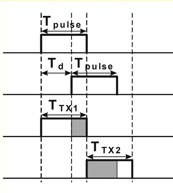
Figure 5 Simplified clocking scheme of a pulsed 3D ToF sensor.
