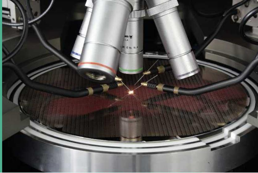
In the new microsystems technology lab (MST-Lab) we integrate different micro- and nanofunctions directly on top of the signal processing CMOS circuits. This procedure is called post-processing. (600 square meters)
