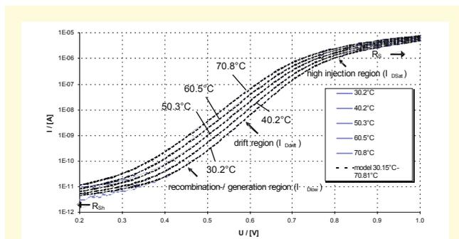
Fig.4: Measured and modeled temperature dependent DC-characteristic
