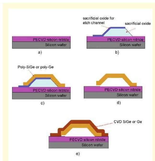
Figure 1: A simplified process flow for the production of the free standing structures sealed with SiGe or Ge. a) dummy wafer with PECVD silicon nitride; b) sacrificial oxide for the spacer of the "capacitors" and the etch channels are deposited and structured; c) poly-SiGe or poly-Ge films are deposited and structured; d) sacrificial oxide is removed; e) "capacitors" are sealed in vacuum using CVD SiGe or CVD Ge.
