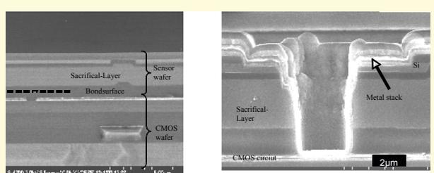
Fig.8: Bonded and grinded sensor- and CMOS-wafer (left), electrical contact between both wafer (right)
