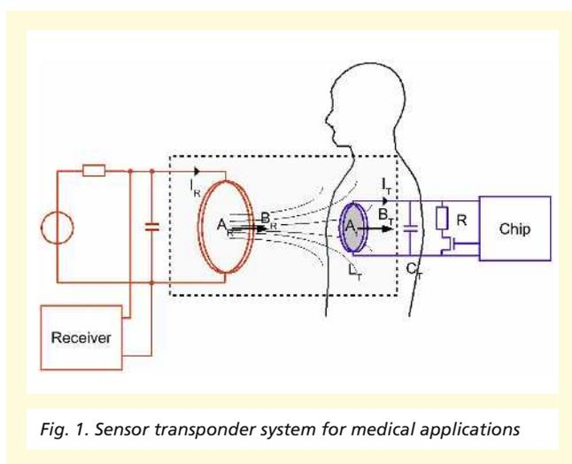
Fig. 1. Sensor transponder system for medical applications
