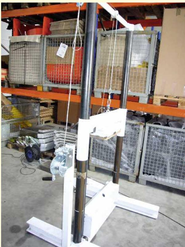
Figure 4: Simulation of Crash Events in the early development phase
