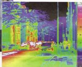
the invisible infrared radiation. The problem is that infrared cameras for the wavelength range above five micrometers like it cold – the sensor has to be constantly cooled down to about minus 193 degrees Celsius. Uncooled imagers for the long-wave infrared range do already exist today, but they are mainly used in the military sphere and are more or less unavailable on the European market. This is now
