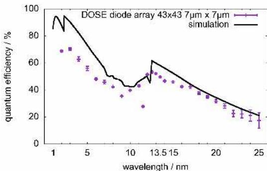
Figure 3: Sensitivity of an array of 43 x 43 DOSE photo diodes with a size of 7 µm x 7 µm compared to a simulation. The quantum efficiency is the amount of detected electron hole pairs divided by the number of impinging photons and the amount of electron hole pairs that are generated per absorbed photon. This amount is calculated using a mean electron-hole pair creation energy of 3.7 eV.
