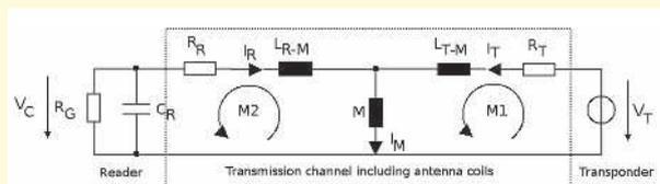
Fig. 2. Equivalent circuit of the load-modulation transmission channel
