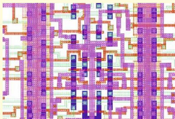
*Fig. 3: Zoomed View of Sinc Filter Datapath. Note the use of polysilicon as routing layer in addition to metal 1 and 2 layers.*
