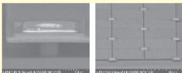
*Fig.10: Contact plug of a diode bolometer (left), array of re-leased diode bolometers (right)*
