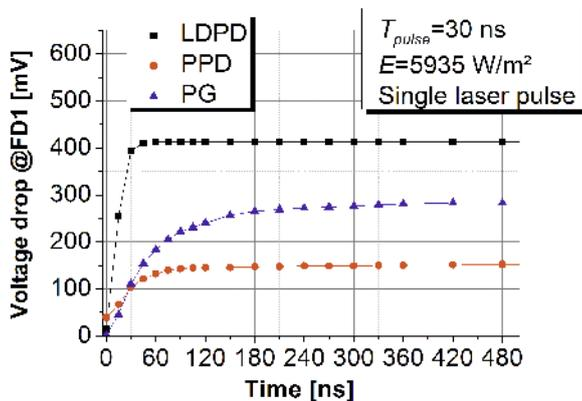
Figure 4 Indirect measurement of the charge collection time in three different pixel structures. ( $T_{LDPD} = 30$  ns;  $T_{PPD} = 60$  ns;  $T_{PG} = 120$  ns).
