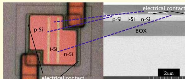
Fig.2: Top view (left) and technological cross section (right) of a SOI-pin-diode test structure
