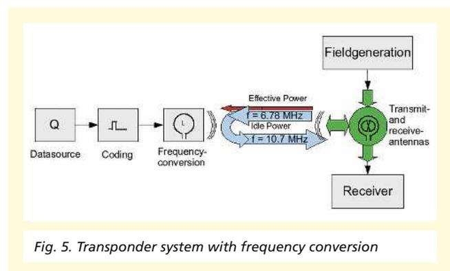
Fig. 5. Transponder system with frequency conversion
