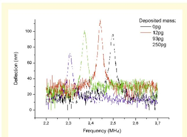
Figure 4: Deflection amplitude as a function of frequency of 96 μm membranes with different silicon oxide masses deposited by FIB. The deflection has been measured by optical interferometry at atmospheric pressure and the excitation is a sinusoidal signal of 3V amplitude.
