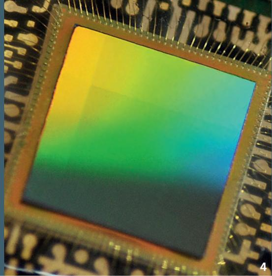
**4** Uncooled IR detector for thermal imaging
