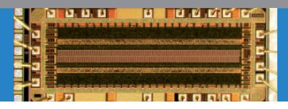
1 Chip microphotograph of SPAD linear sensor
