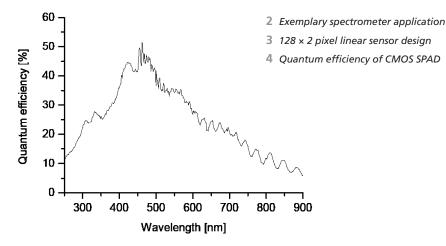
All these applications are characterized by the requirement of counting single photons in order to acquire the intensity and the shape of the optical wave carrying very weak signal information under real-time measurement conditions. In order to increase the resolution even further and capture ultra-fast events in the picosecond regime, the photon arrival time-stamp is repetitively time-correlated by employing histogram binning analysis method.
