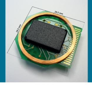
15 cm. As external components for the ASIC, only an antenna based on a coil with a resonance capacitor and an additional capacitor for smoothing the operating voltage are necessary, reducing cost and increasing reliability of the system (Figure 4). The sensor is calibrated in a fully automatic way, storing the calibration coefficients for pressure and temperature in the onchip and system EEPROM.
