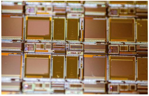
SPAD sensor chips are implemented in CMOS technology. © Fraunhofer IOSB | Picture in color and printing quality: www.fraunhofer.de/en/press
