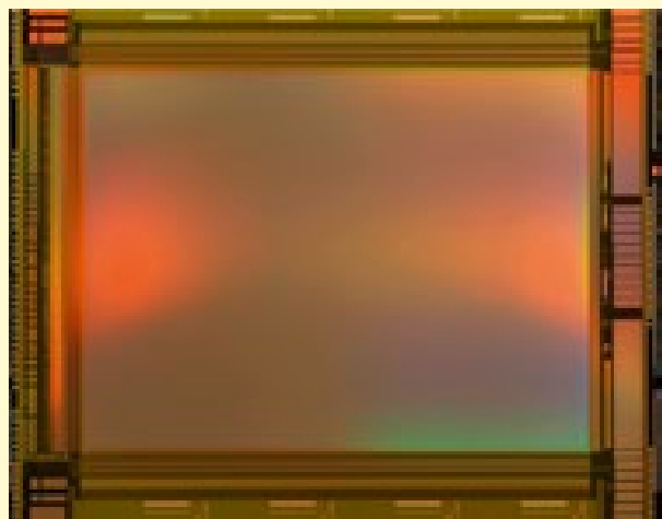
Figure 2: Micro-photograph of the 19.8 mm \times 18.7 mm fabricated high frame-rate HDTV sensor.
