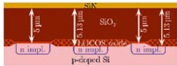
Figure 3: Schematic of the three investigated photo diodes. A photodiode under thin gate oxide (left), under thick field oxide (middle) and a photodiode according to the proposed structure with half of its area under thin and the other half under thick thermal oxide (right) is shown.
