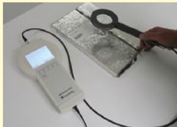
Figure 1: Readout of the inside pressure and temperature of a VIP
