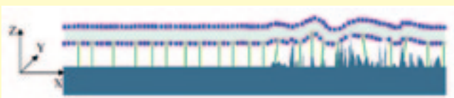
Figure 4: Schematic representation of the effect of surface roughness on tBLMs. [3]
