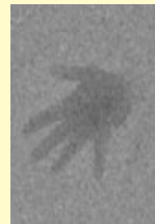
Figure 10: Uncompensated IR image with f/1.2 optics
