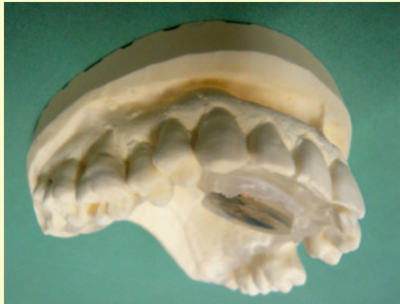
Figure 1: In silicone encapsulated telemetric pressure sensor fixed to an imprint of the hard palate that is placed on a model of the upper jaw.
