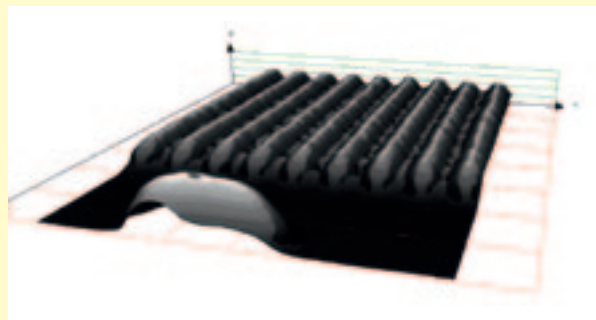
Figure 8: Shape of cylindrical micro lenses (pitch = 6\ \mu\text{m} ) measured using a phase shift microscope
