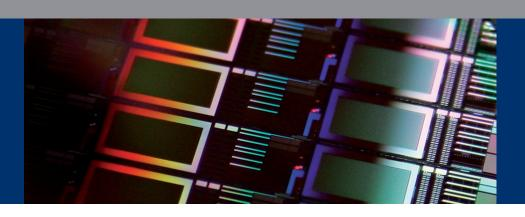
1 CSPAD3000 on wafer level
