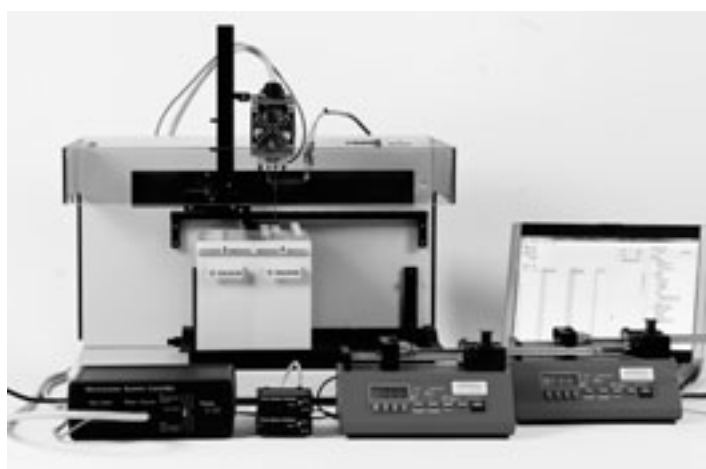
Figure 3: Picture of the automated Micro-Reactor setup to optimize industrially relevant reactions. This system can be used as an initial screening before large scale optimization saving costly chemicals.
