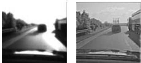
Comparison of images taken with CCD (left) and CMOS (right) cameras
